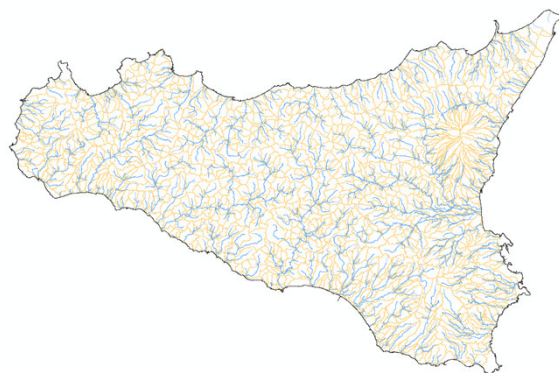
Figure 3: Derived Drainage Network and Catchment Delineation (Stream Definition: 10 km 2 )
